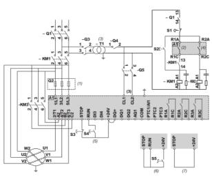
(1) : Installation of additional fast-acting fuses to upgrade to type 2 coordination according to IEC 60947–4–2.
