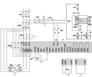
(1) : Installation of additional fast-acting fuses to upgrade to type 2 coordination according to IEC 60947–4–2.
