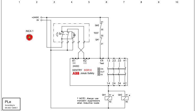
Note: The stated PL is only valid if all relevant requirements according to EN ISO 13849-1/-2 are met. It is the responsibility of the machine builder to make a risk assessment and make sure that the appropriate functional safety levels are achieved.
